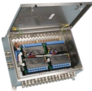
Intrinsically Safe Multiplexer system
